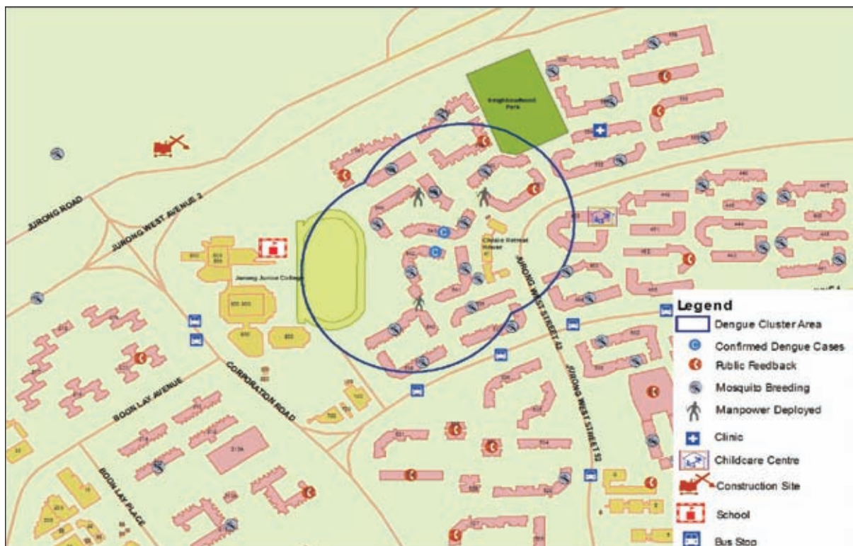
Figure 16: Planning, managing and deploying resources for vector control operations using GIS
